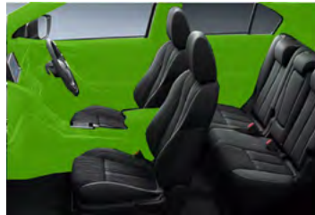
Main parts (indicated in green) that use thermoplastic resin on the Eclipse Cross . Top: Exterior, Bottom: Interior
