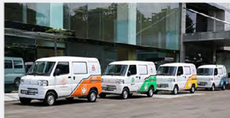
"MINICAB-MiEVs," Kei-car segment commercial battery electric vehicles, being used in a pilot study (Indonesia)
