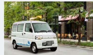
The “MINICAB-MiEV” is a one-box-type vehicle that incorporates the EV systems of the “i-MiEV,” which has a proven track record in the world’s first mass-produced electric vehicle. This system includes a drive battery and a small, lightweight and highly efficient motor. We have paid careful attention to the layout of the EV components, such as the drive battery, resulting in a spacious cargo area, as well as excellent driving stability and comfort thanks to a low center of gravity.
